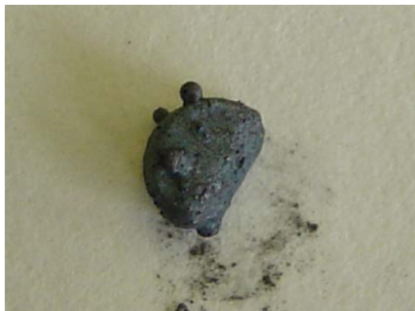
Figure 1 Photograph of pellet of sample 4 following the SHS reaction showing significant deformation of the pellet.
